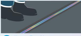
Narrow Trenching Creating a very narrow cut (approx. 12mm) in a hard surface (such as concrete) usually following an existing join, installing the fibre
